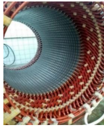
Figure 10 – Partial view of the stator winding (Villibor et al., 2022).
